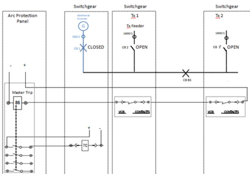
Fig. 5.5 DG isolation scheme for two transformer feeders in OFF status.
