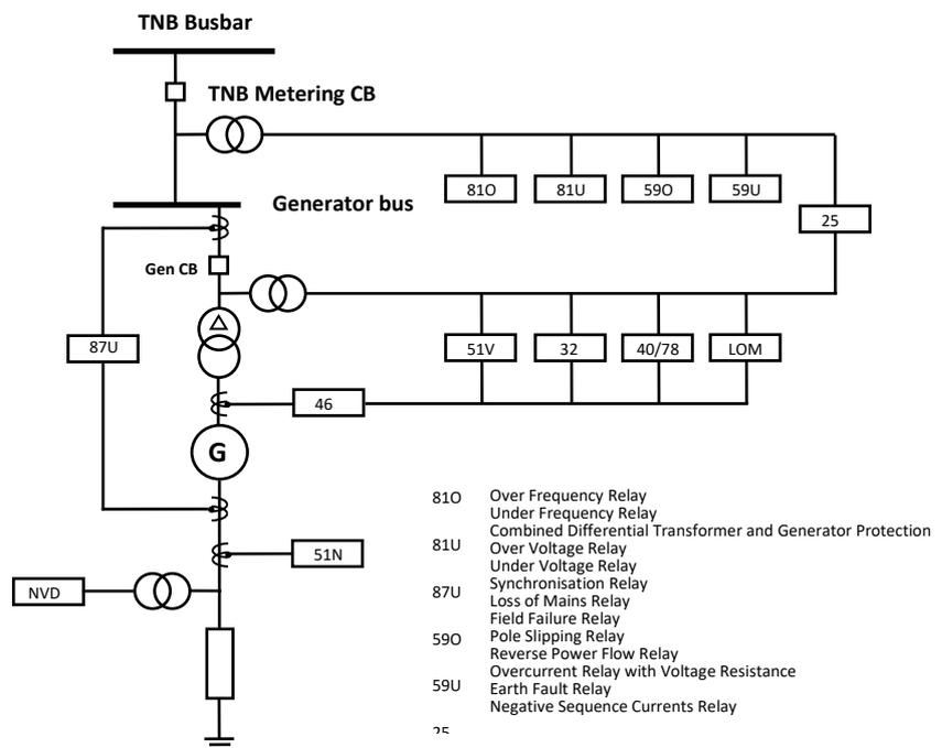
Fig. 5.1 Distributed Generator protection schemes.
