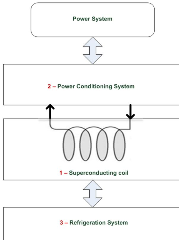
Fig. 2.7 Superconducting Magnetic Storage Systems' Components.
