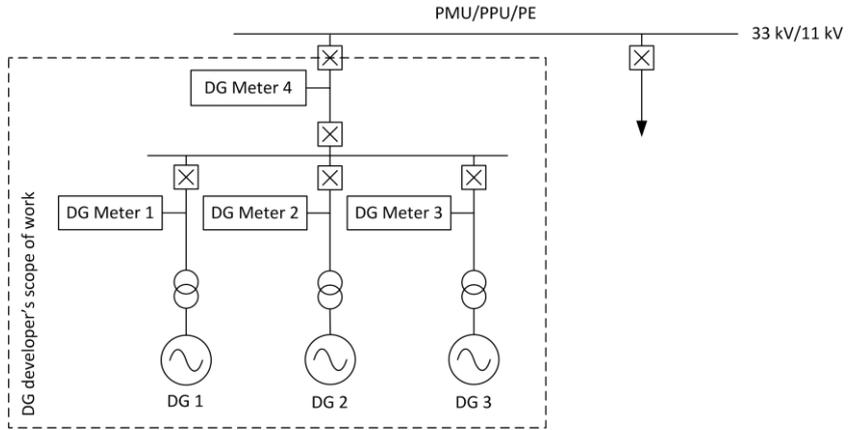
Fig. 3.8 DG connections for MV output at PMU/PPU/PE (direct multiple-feed connection).
