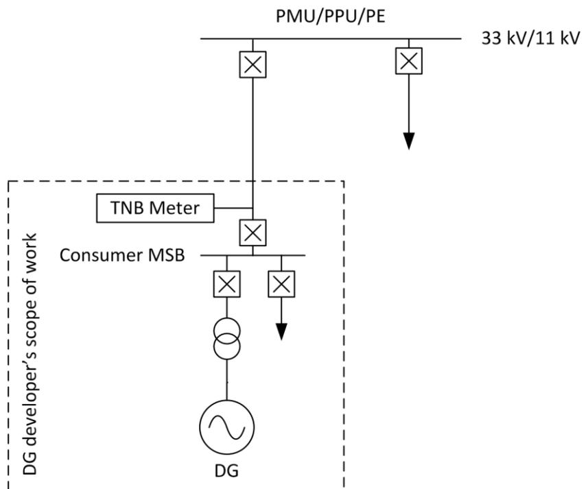
Fig. 3.7 DG connections for MV output at PMU/PPU/PE (indirect connection).
