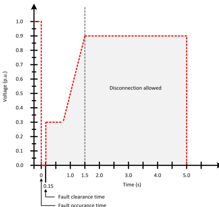
Fig. 4.1 Operation of LSS during system voltage fluctuation.
