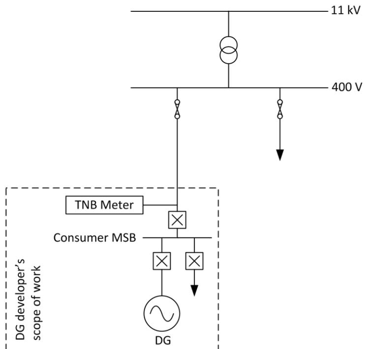
Fig. 3.5 DG connections for single-phase and three-phase LV (indirect connection).
