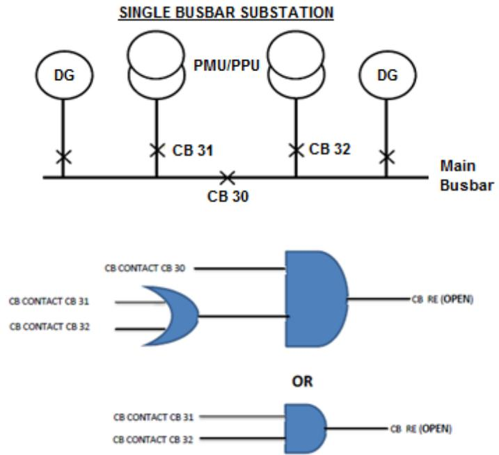
Fig. 5.6 DG Isolation Single Line Diagram and logic.
