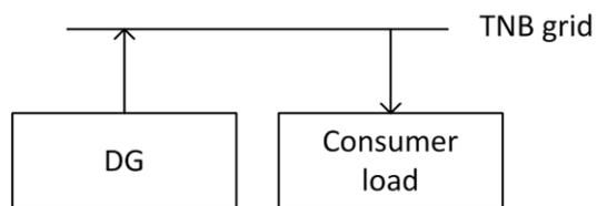
Fig. 3.1 Connection to TNB grid (direct).
