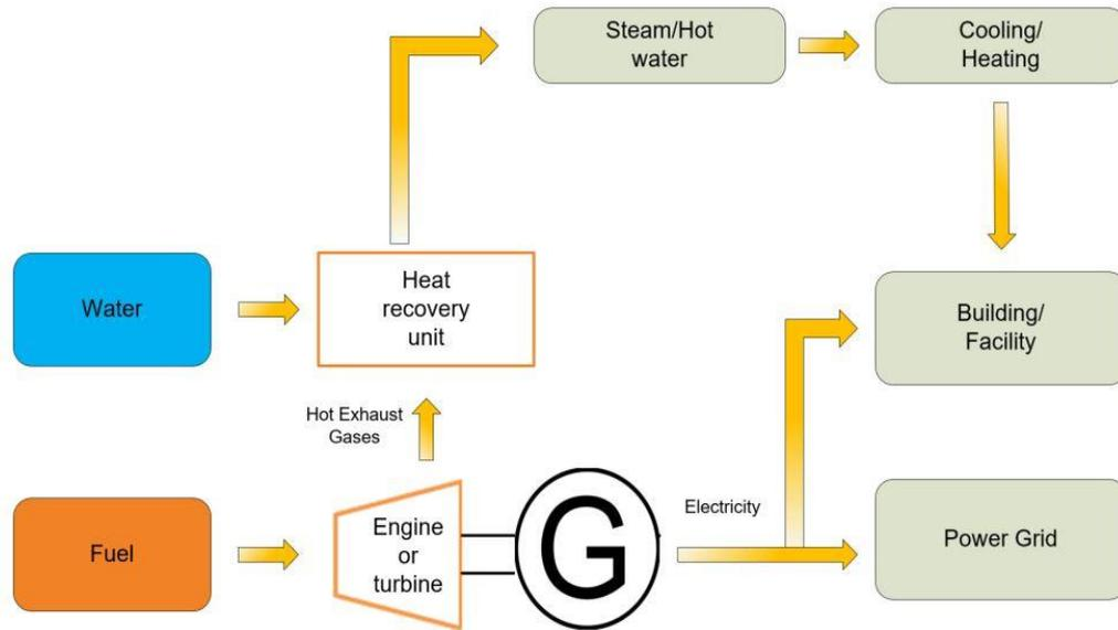
Fig. 2.5 Schematic of Combined Heat and Power (CHP) plant.
