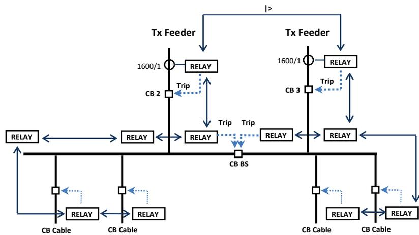
Fig. 5.3 Arc Protection Scheme without RE.
