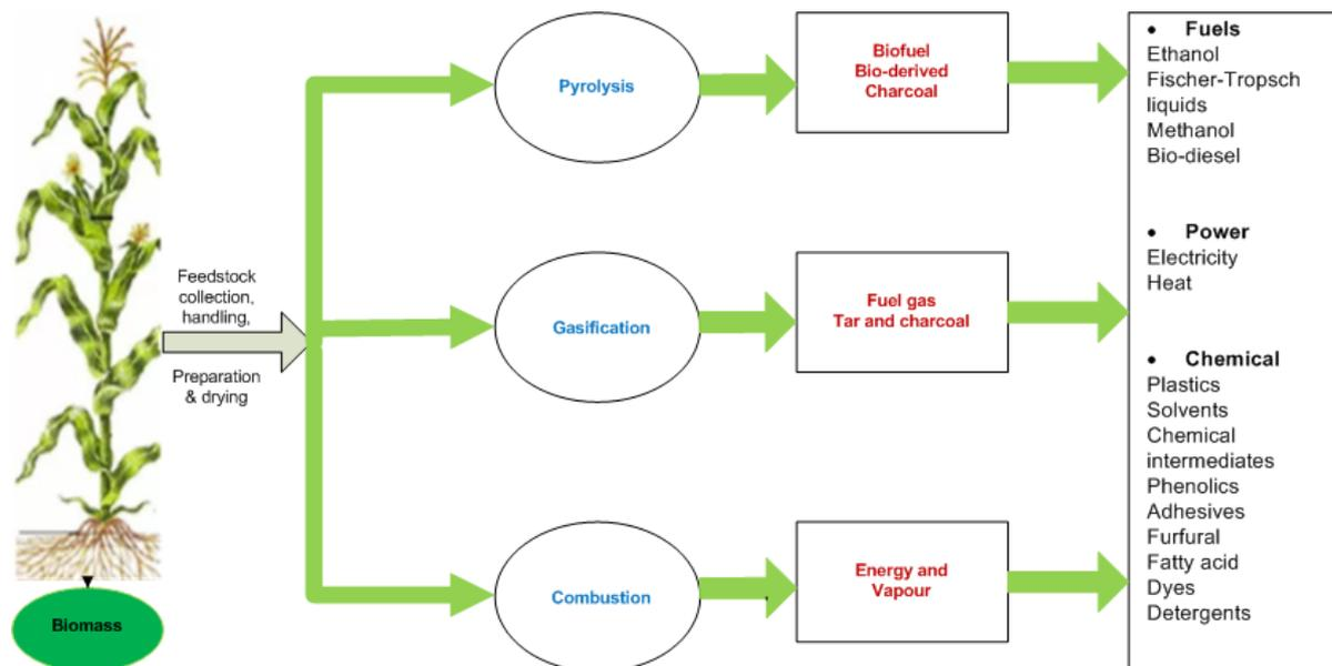
Fig. 2.4 Thermochemical Conversion Technologies for Biomass.
