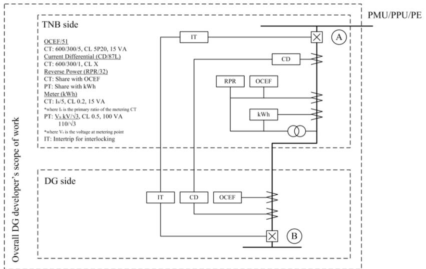
Fig. 3.9 Interconnections diagram between TNB and DG.
