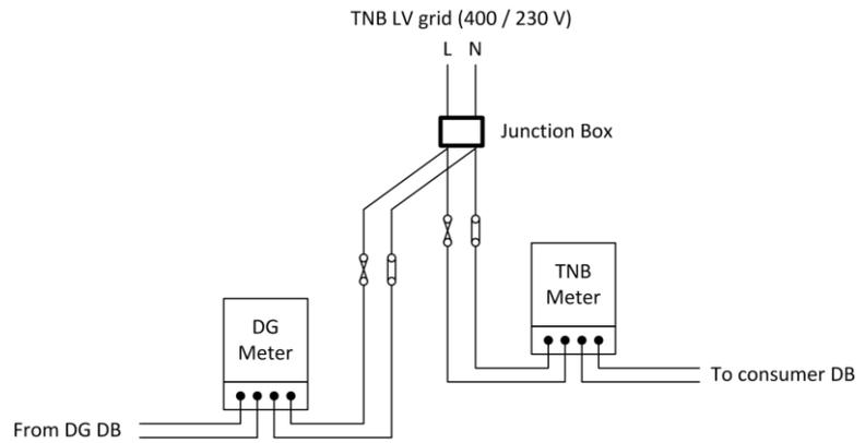
Fig. 3.4(ii) DG connections for single-phase and three-phase LV (direct connection).
