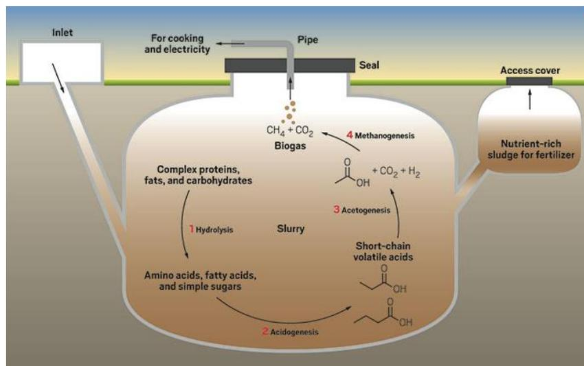
Fig. 2.1 A simple anaerobic digester where different bacteria break down the waste that is loaded inside in four stages [13].
