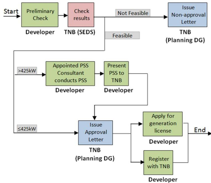
Fig. 9.2 Application Process Flow for Indirect Connection (Selco & COGEN) to TNB.
