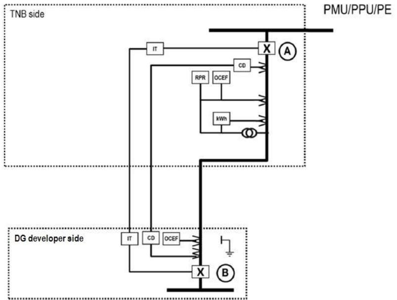
Fig. 5.9 Interlocking of the interconnection feeder with TNB.
