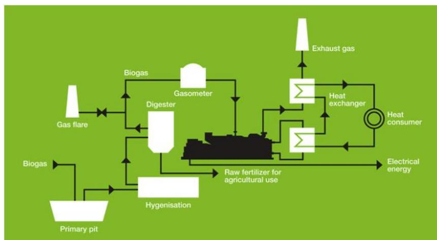
Fig. 2.2 Biogas cogeneration flow diagram.
