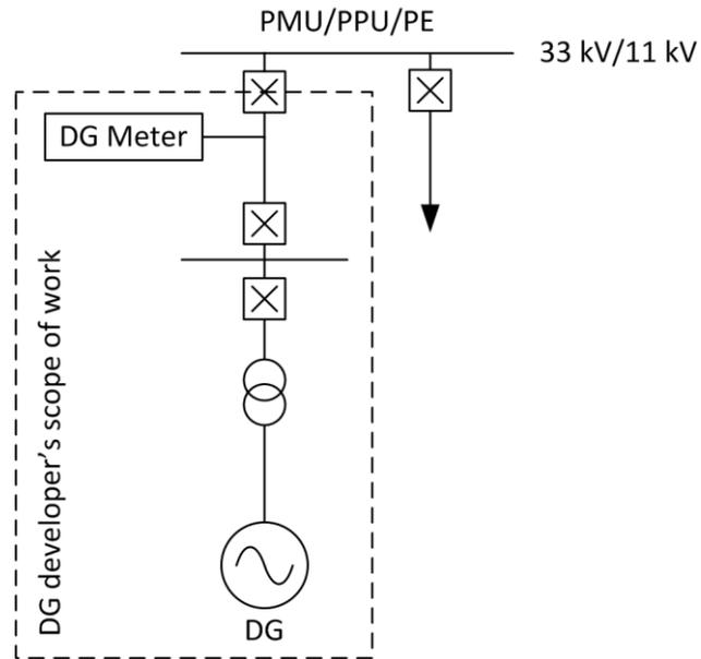
Fig. 3.6 DG connections for MV output at PMU/PPU/PE (direct connection).
