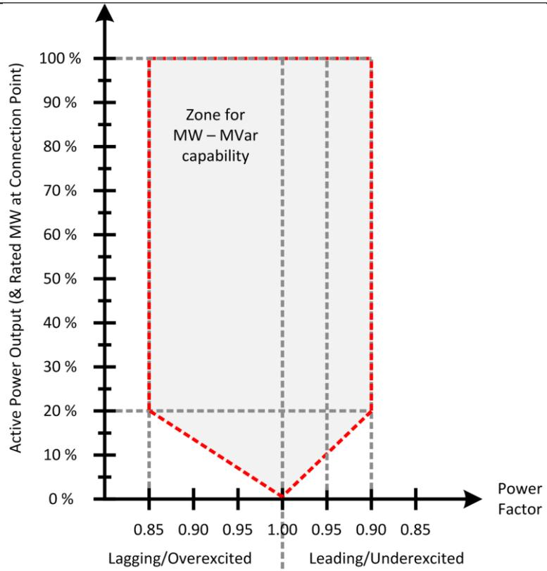
Fig. 4.3 Reactive power requirement at connection point for LSS.
