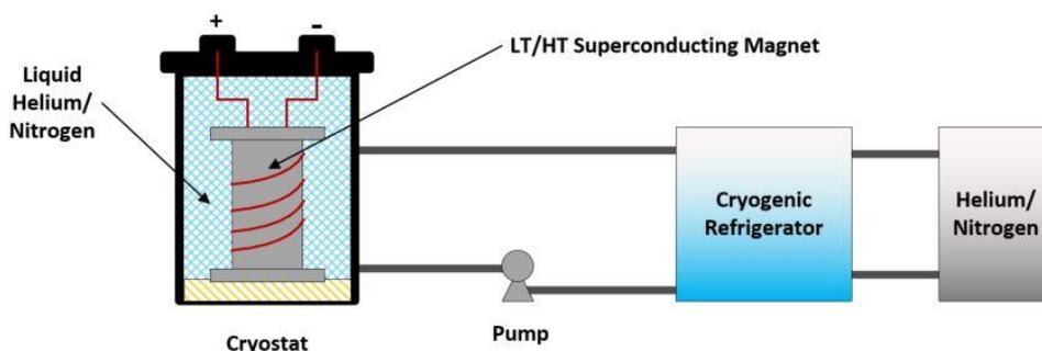
Fig. 2.8 Schematic diagram of SMES [23].
