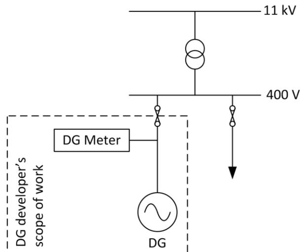
Fig. 3.4(i) DG connections for three-phase LV (direct connection).
