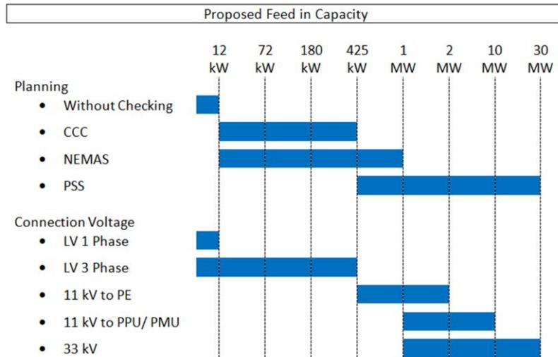
Fig. 3.3 Planning process and point of connection based on proposed DG output.
