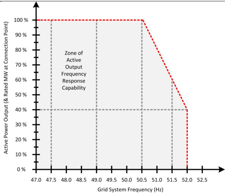
Fig. 4.2 Active power output versus frequency.
