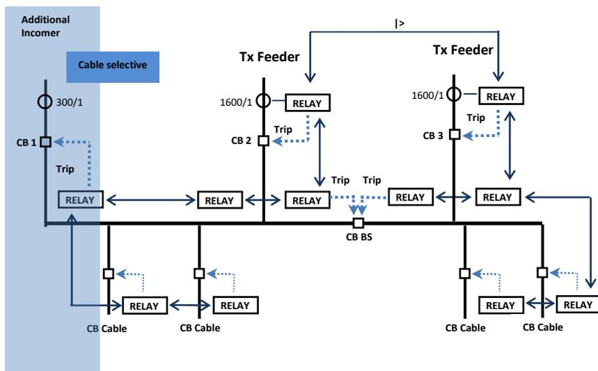
Fig. 5.4 Arc protection with RE.
